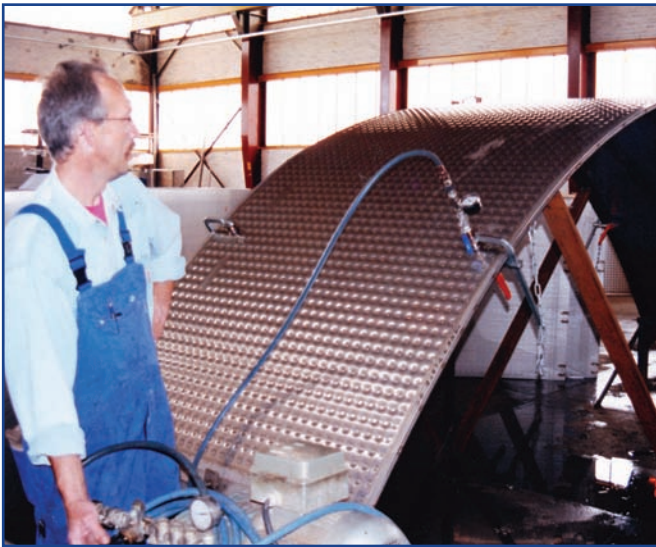
Left: Inflating clamp-on cooling panels. Right: Top of existing 5275 kW (1,500 ton) \text{NH}_3 separator to be retrofitted to 12 309 kW (3,500 ton) separator.
